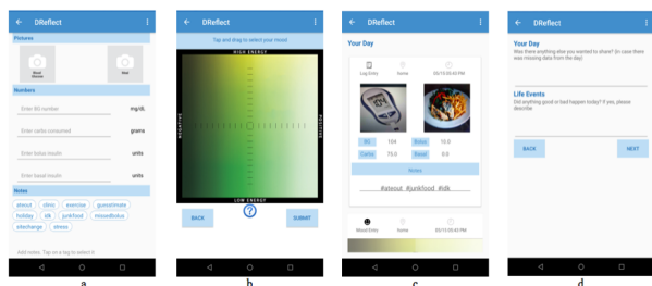
Figure 1: The DReflect System a) meal log screen, b) mood report screen, c) end of day data summary, and d) end of day questions
